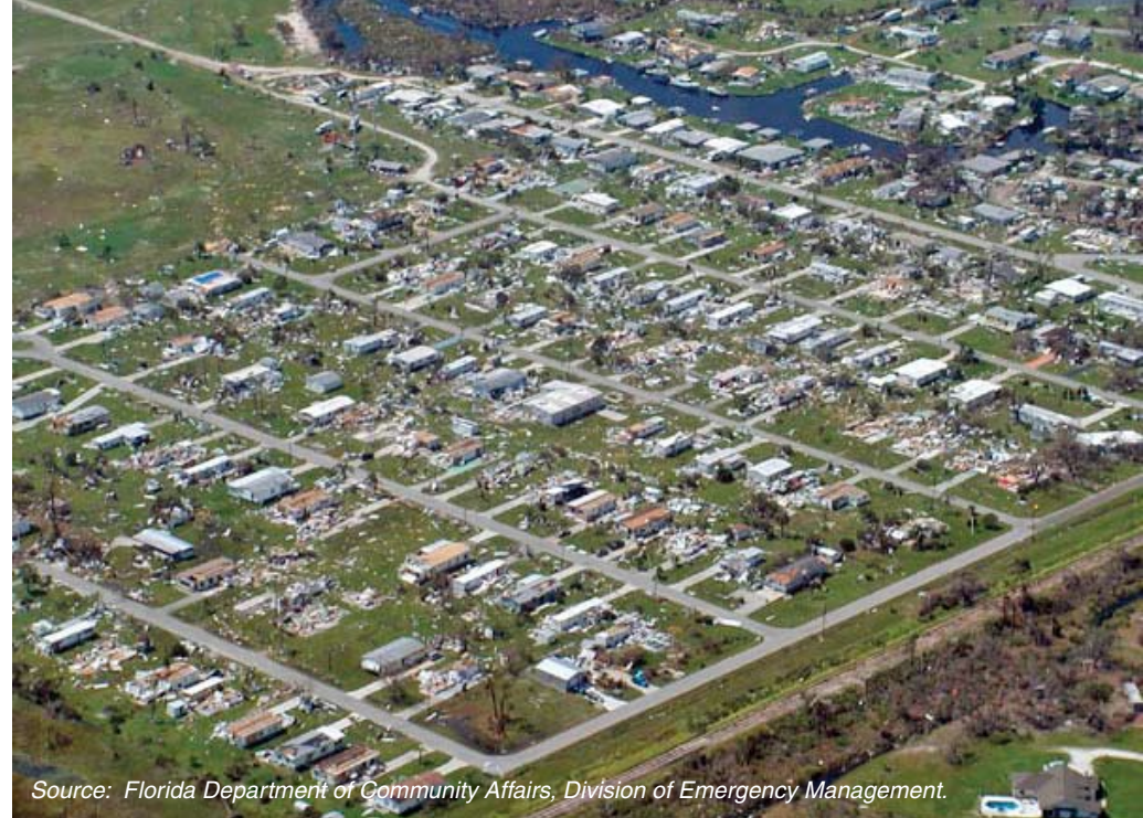
Figure 5.10: Mobile home wind damage from Hurricane Charley.
